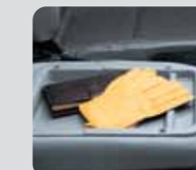
Center seat back tray: The back of the center seat converts into a tray when folded
